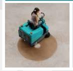
The compact ASC EUREKA M2 sweeper has a reduced turning radius (950 mm), which enables cleaning in tight spaces which are difficult
