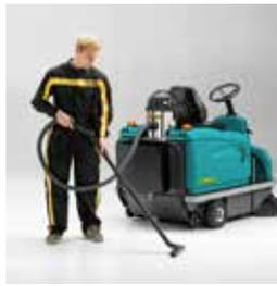
The ASC EUREKA M3 sweeper (EB version only) is also available with a vacuum cleaner kit. Designed for cleaning under tables, chairs, and other recesses or to reach shelving and raised surfaces.
