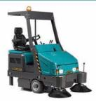
The ASC Eureka M6 is a completely hydraulic controlled high dump sweeper.
